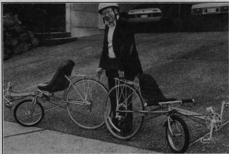
John Dusenberry with his original and 1984 chrome Hypercycles. Both have inverted seat posts used as front der. posts. (photo by Jon Schwartz)
