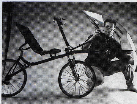
The Presto SE with optional Zipper fairing & suspended fork photo courtesy of Angle Tech
