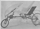
The ATP Vision R-40 LRS with LRS, 17" front wheel and an ATP zipper front fender.
