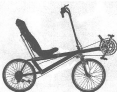
An artist's conception of the Angletech full suspension Affluence with Boulder rear suspension, ballistic front suspension, Flare seat, Flip-Fit stem, dual 20" wheels and CHMS frame pipe (3' and Alarm, available)
