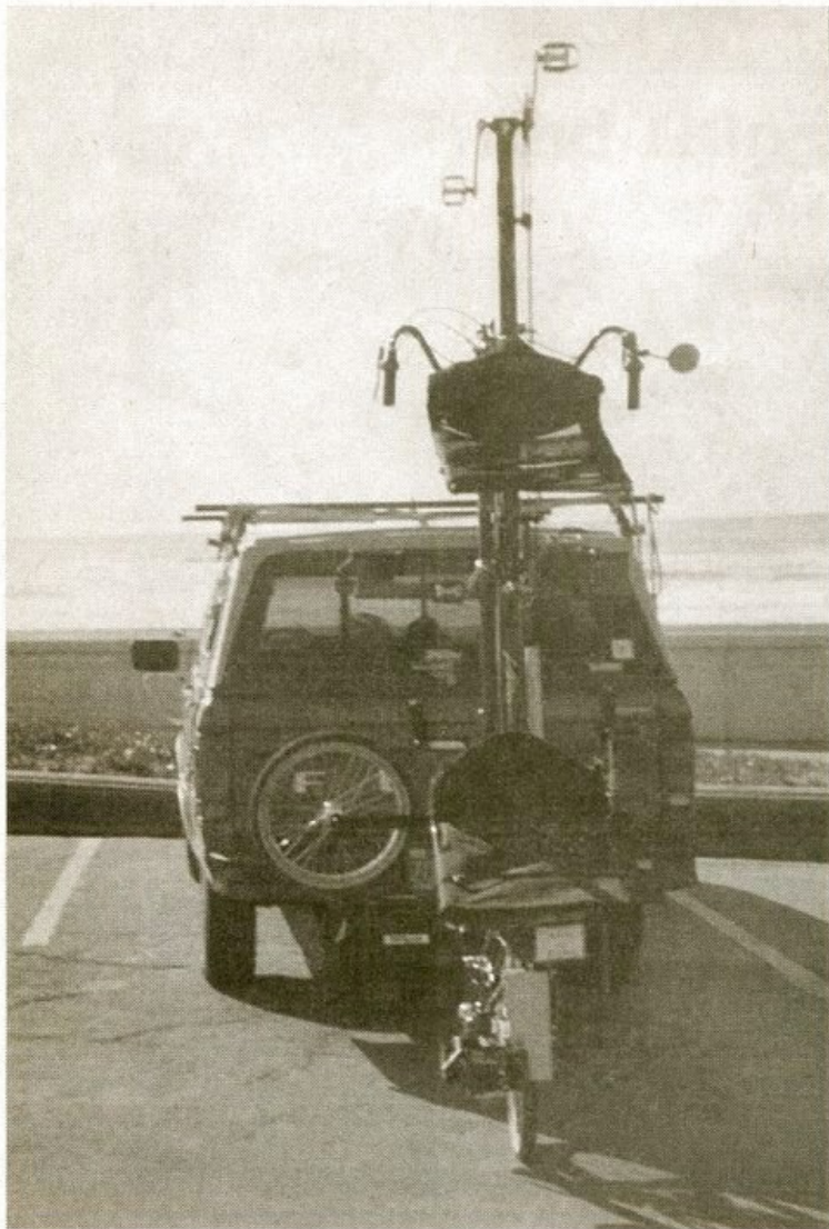
Vision tandem attached to rack and sitting on ground. Next step is to push forward on central bar and entire system will close up next to the truck. Locking pin is inserted.
