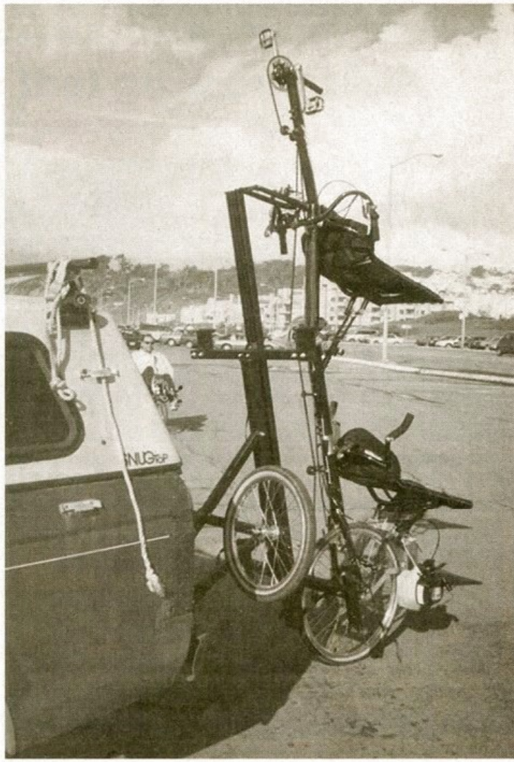
The DraftMaster system attached to the truck's hitch receiver, balanced on the tandem accessory rail base, with one 20" front wheel attached. It stores in our garage just as it is, until our next outing.
