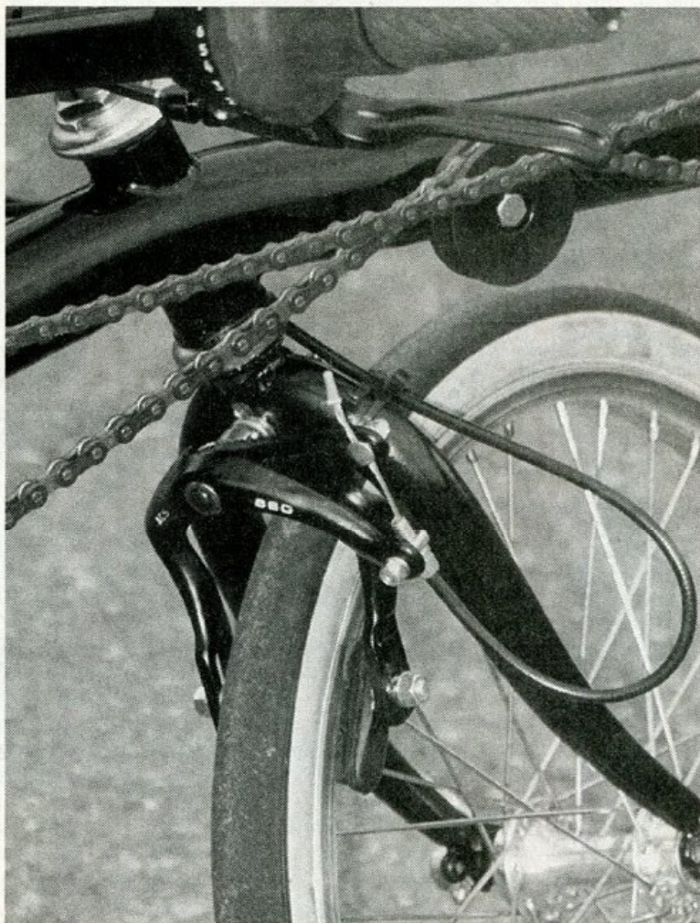
The T-Lite's wacky front brake cable routing and noisy bearingless chain idler. Both are badly in need of updating.
