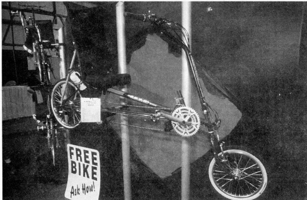
The $695 Rans Wave compact. This bike is very similar to the Tailwind, though it has lower line components, lower gearing, shorter wheelbase and a 16" front wheel.—John Riley
