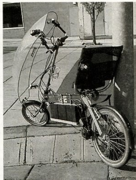
RIGHT: Bike Cockpit from L to R, Night Rider Light, Wes in Mirror, Left hand thumb motor engagement control, Right hand thumb hi/low light switch, Right hand finger electric throttle (hold down) hi/low switch. Night Rider Light mount is removable and can be used as a spotlight.
