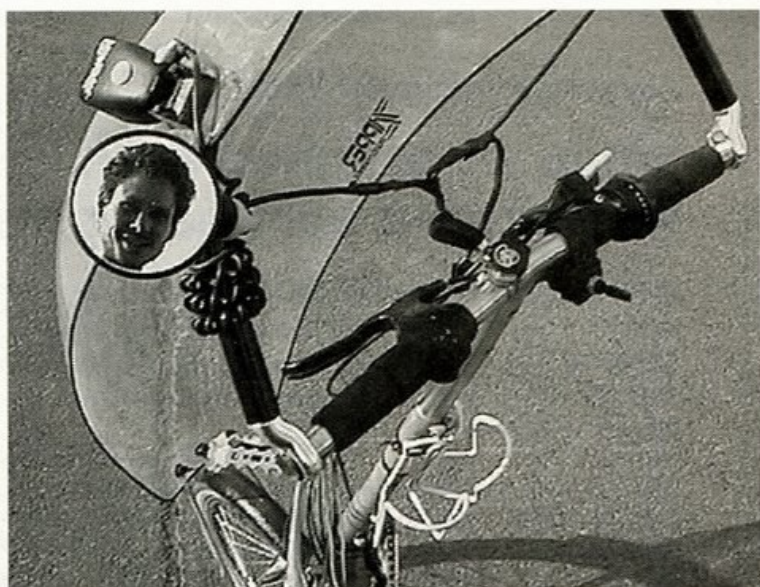
RIGHT: Bike Cockpit from L to R, Night Rider Light, Wes in Mirror, Left hand thumb motor engagement control, Right hand thumb hi/low light switch, Right hand finger electric throttle (hold down) hi/low switch. Night Rider Light mount is removable and can be used as a spotlight.
