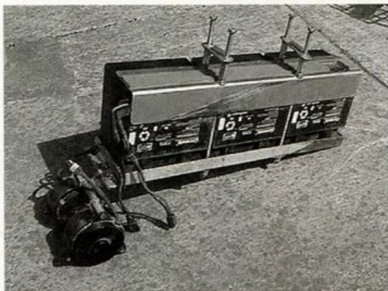
BELOW: motor is mounted at rear to aluminum welded frame holding batteries. Aluminum Plate covers battery wiring. Size 20 bolts mount unit to frame and hold batteries in place when dismantled
