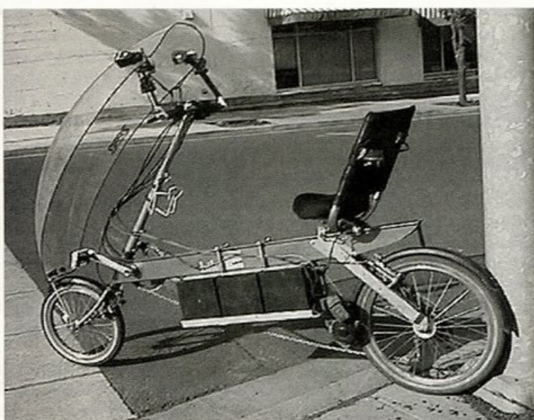
Note dual Night Rider lights mounted above fairing, dual WB cages and cut off frame tail
