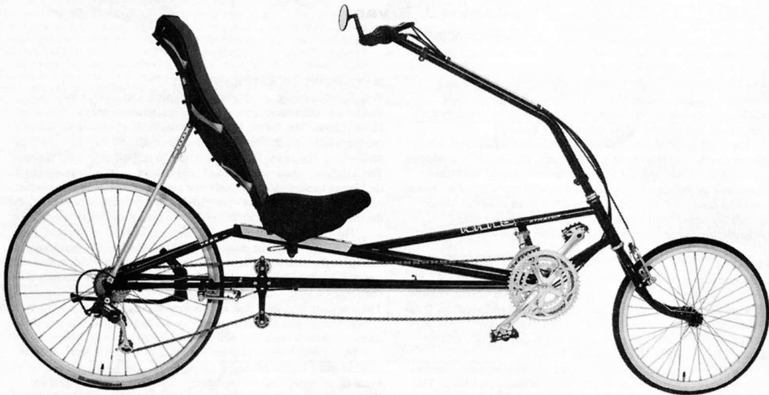
The 1999 Rans Stratus—a wonderful classic long-wheelbase (LWB) above-seat steering (ASS) recumbent. This model is tried and true—the flagship of the Rans line. The Stratus offers superior comfort, performance and style. Most owners will be set for life. We love this bike.—photo courtesy of the Rans company.
