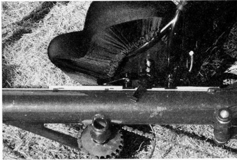
Trek mainframe and back side of mid-drive. Note Trek seat track with Rans seat.
