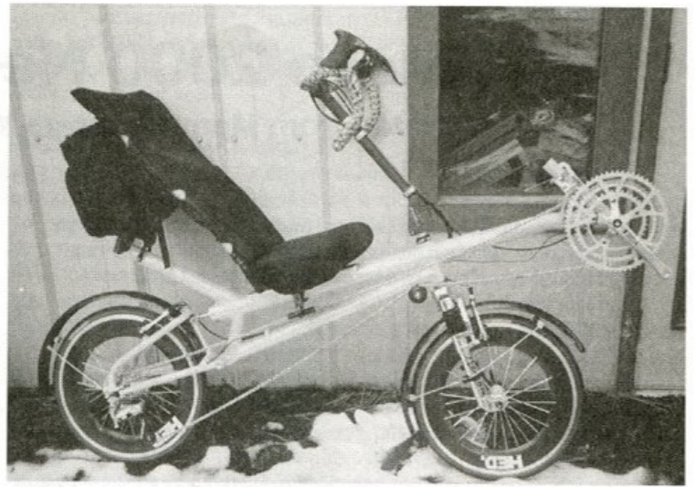
The 2000 Angletech Altitude SHO full suspension SWB ASS with drop bars, HED wheels and a host of hitch goodies. This is the best suspension SWB made
