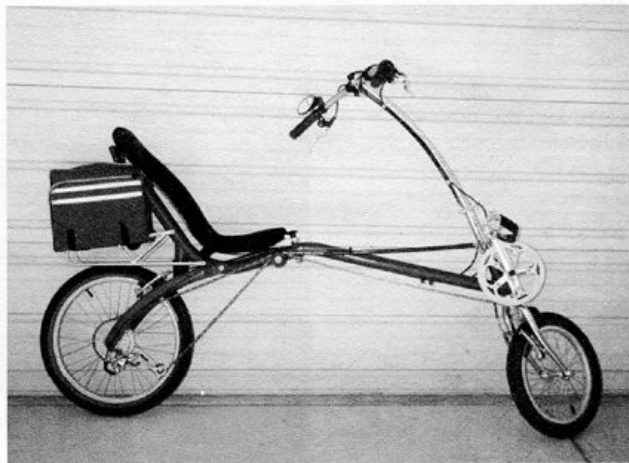
M5 Compact—note hinge just ahead of seat
