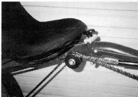
M5 Compact folding hinge
