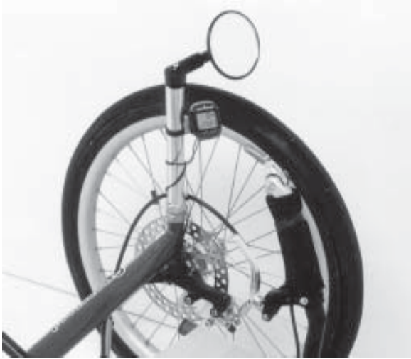
Note optional disc brakes, computer/mirror mount and our favorite bar-con bar-end shifters
