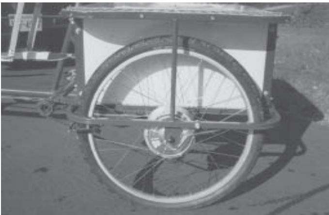
The Transporter's electric assist/drive wheel. The other side has an electric assist too, but is not a drive wheel.
