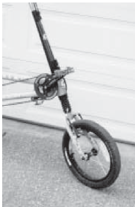
Above: The Easy Rider's rear suspension Below left: The Cannondale HeadShok for a 305 mm front wheel
