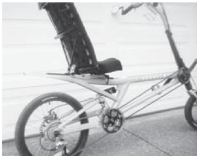
Above: The Easy Rider's rear suspension Below left: The Cannondale HeadShok for a 305 mm front wheel
