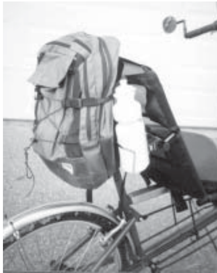
Lightfoot rear seatpost forks allow for recline adjust and keep the seat from slipping
