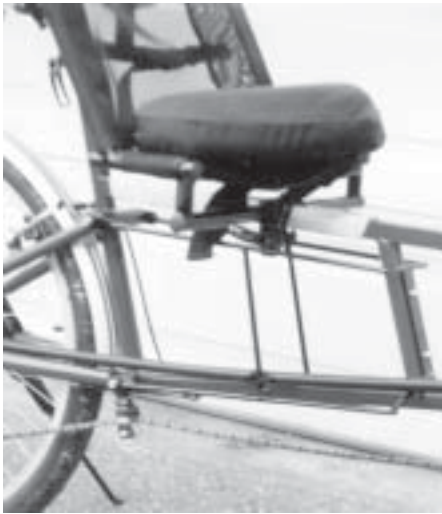
Note underseat CroMoly pannier rack (holds four panniers)
