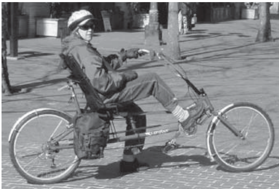
The Ranger as an urban commuter. The underseat pannier rack will take two panniers on each side. We also strapped our trusty L.L. Bean backpack to the seat back with one bungee cord. This bike can haul lots of stuff.
