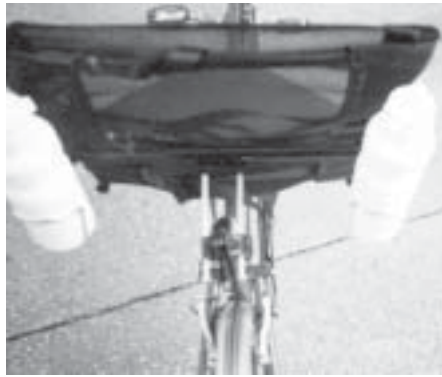
Lightfoot rear seatpost forks allow for recline adjust and keep the seat from slipping
