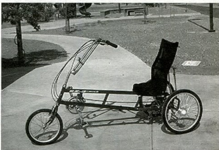
The EZ3 has twin 20-inch (406 mm) rear wheels and a 16-inch (305 mm) front wheel. The new 2003 aluminum version will have 3 20" wheels. This will not be a second model. Much like the EZ1 SC Lite is to the EZ1 (Rick Higginson)
