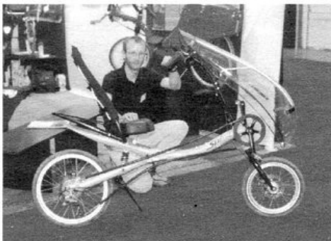
Paul Hollants and the HP Velo Spirit dual suspension compact LWB with fairing (John Riley)
