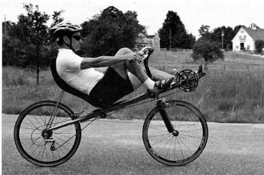
Side view of Rich Pinto on the Bacchetta Aero. Note that the bars, as well as the circle made by the rider's legs, are sheltered within the area swept out by the rider's body. (Photo Copyright © 2003 Randy H. Goodman)
