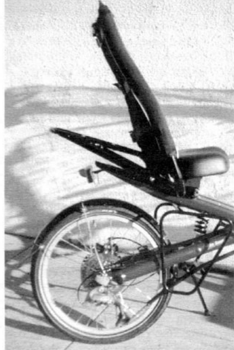
Note the Spirit's seat, integral luggage rack and optional pannier rack. The seat has better recline and angle adjustment than most CLWB models.
