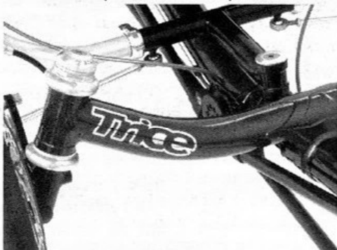
Trice steering pivots on Stronglight headsets
