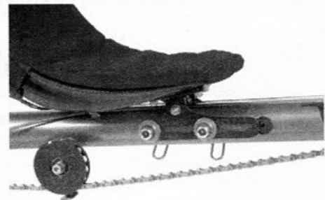
The seat mounts go through the main frame via a small tube in between the mainframe tube. Note Greenspeed idler.
