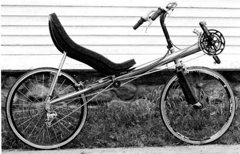
The 2003 Bacchetta Aero will include an improved design for the bars and the seat/idler mount over those pictured, and will ship with bladed Velocity Pro wheels resembling the rear wheel shown. The frame will also be available in two sizes, to accommodate taller riders. (Photo Copyright © 2003 Randy H. Goodman).
