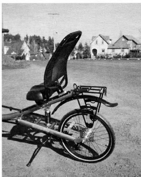
Scooterbike rear end: note extreme lumbar in seat, cool rack and rear fender mounting — RCN photo
