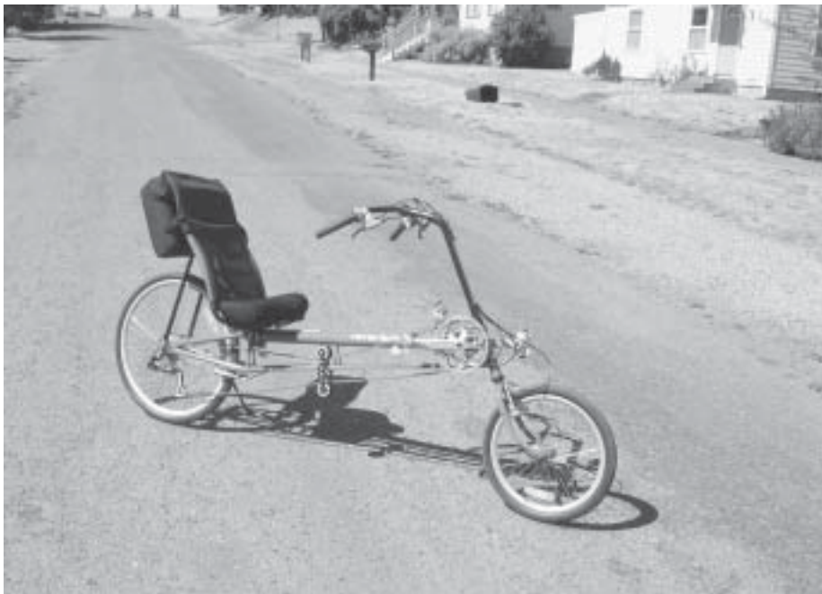
The RANS V2 is an exceptional buy at $1,299. The high BB and double bend handlebar steering isn't as user-friendly as other LWB OSS recumbents.
