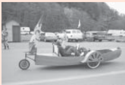
Autocanoe — This new rear-wheel steering, front-wheel drive tadpole trike will keep you cool, because it's amphibious. Head for any boat ramp for a seamless transition to recumbent canoe. See page 4
