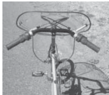
Note the fairing shape in this photo. The Mueller mounts work very well on the Stratus. This bike has the mid-reach B-33 stem and B-36 single bend bars.
