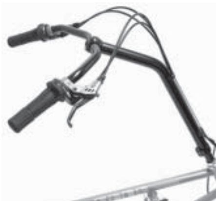
This is the stock 2004 Stratus bar/stem combo. Shown is the B-32 mid-reach stem and B-37 double bend bars.
