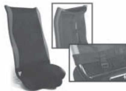
The updated RANS seat back is comfortable and refined. Gone are the zip ties, replaced by adjustable buckles.
