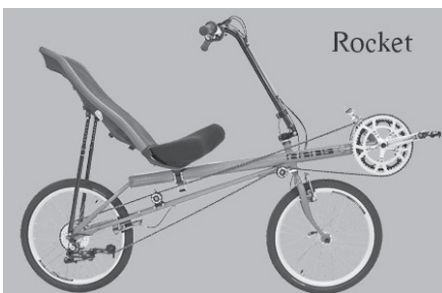
The 2005 RANS Rocket has an X-7 drivetrain and a Truvativ Elita crankset and sells for $1174 — oh yes, and it's red.
