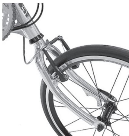
The V2 Formula is sporting a new aluminum fork, with disc brake mounts, (the frame has always had rear disc mounts). The V2 Formula's price is now $2,395.
