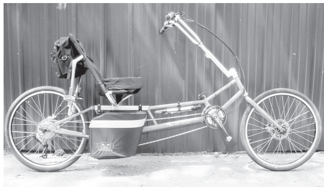
A Lightfoot Rangler with Angletech's GL81 Sram Dual Drive set up — Angletech
