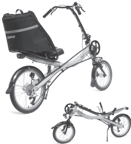
The HP Velo Spirit has a new folding OSS unit, new optional bag, as well as new spec and price for 2005
