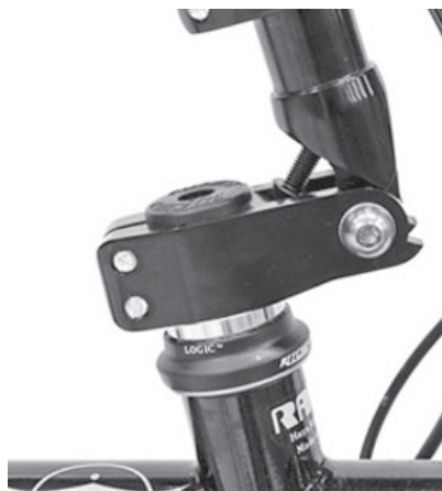
RANS has updated the Flip It for 2005, with wear washers at the hinge and a bolt has replaced the QR for a cleaner, smoother operating Flip-it (all models except Screamer Sport)
