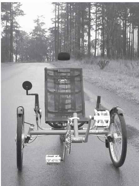
Note the straight cross-member, high seat and relatively low bottom bracket
