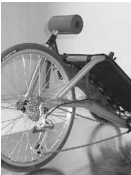
Note the low slung frame, integral seat and clamp-on spring loaded head/neck rest — Photo courtesy of Catrike
