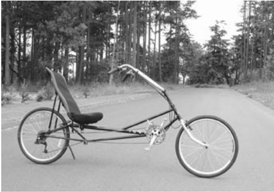
This is our prototype RANS Stratus XP XL. The main change on production models is that the top tube comes rearward towards the seat four more inches.
