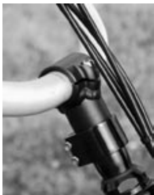
This is the stem piece for the chopper bars. It does not adjust vertically.
