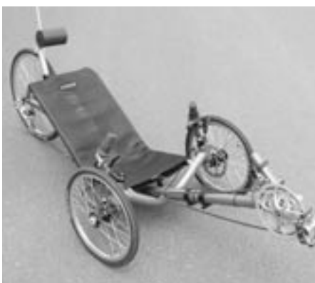
Note the formed frame cross-member that allows the trike to sit so low. Also note head/neck rest mount. Mount on photo below is current.
