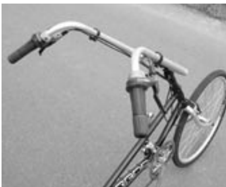
The new RANS chopper bars. Note the telescoping bars (2)
