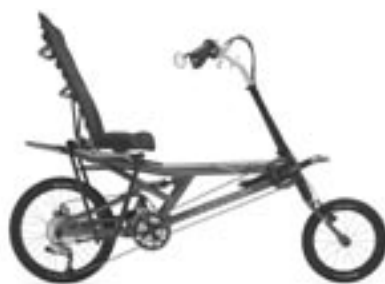
Compact Long Wheelbase: Cannondale Bent 1 dual suspension CLWB
