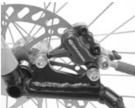
The Gator 4-pot disc brake caliper. This is a hydraulic brake.
