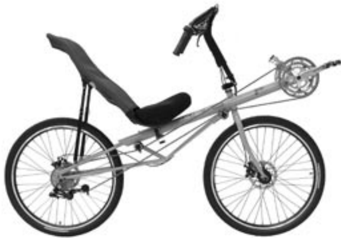
The RANS Force 5 Enduro takes fat 26" or skinny 700c wheels/tires
