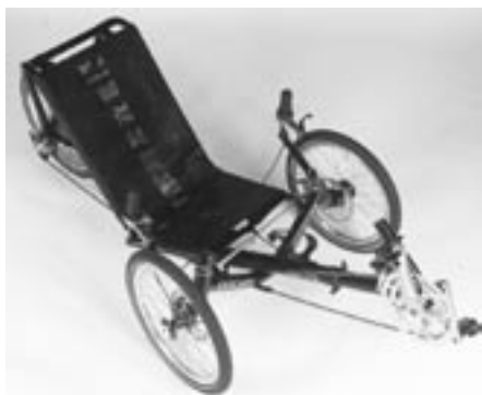
Catrike's 2006 Pocket with 355mm 18" front wheels and a 20" rear wheel
