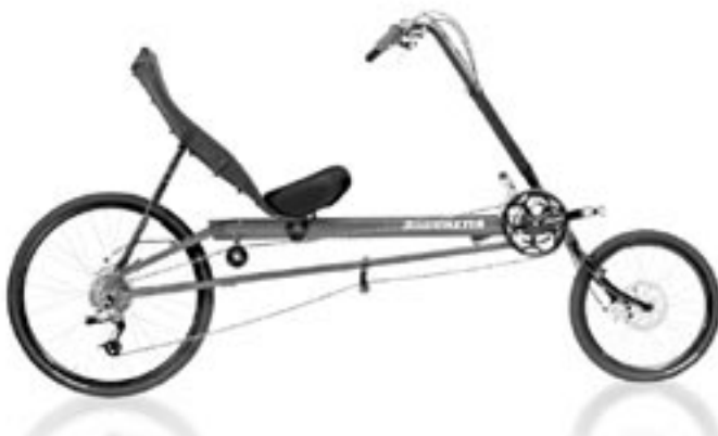
ABOVE: 2006 Bacchetta Agio with aluminum frame and disc brakes
