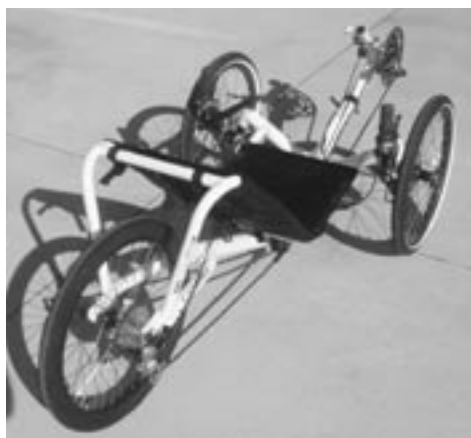
ABOVE: 2006 Bacchetta Agio with aluminum frame and disc brakes
