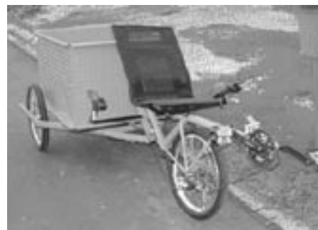
The Organic Engines SUV will haul 500 pounds of cargo and a 250 pound rider
