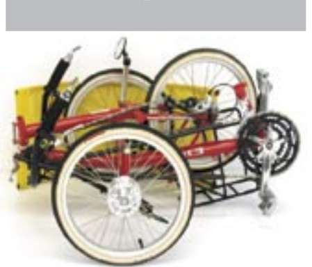
Catrike's 2006 Pocket with 355mm 18" front wheels and a 20" rear wheel
