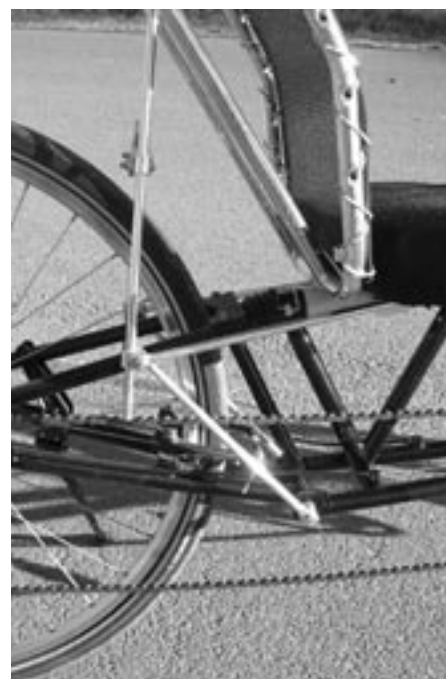
The Fold Rush suspension, swing-arm and seat braces (swing arm bolt/hinge is where lower brace attaches)
