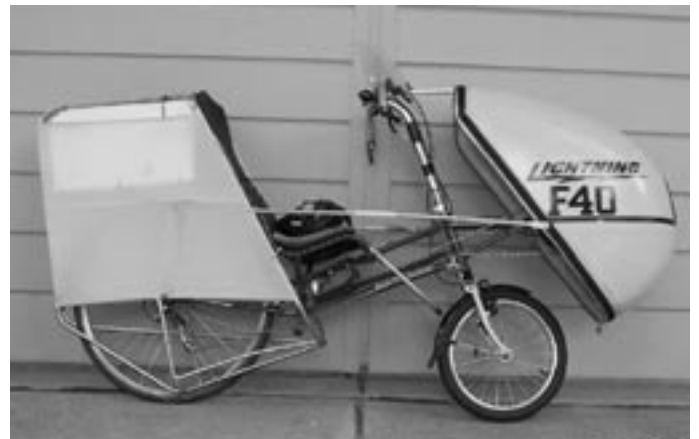
The F-40 is a P-38 chassis with a fiberglass nose cone (front) and aluminum body work (rear)
