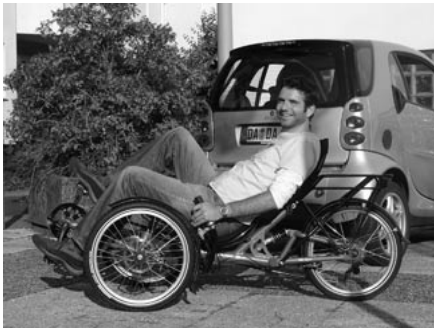
The Scorpion FX has a slightly higher seat and a lower bottom bracket.
