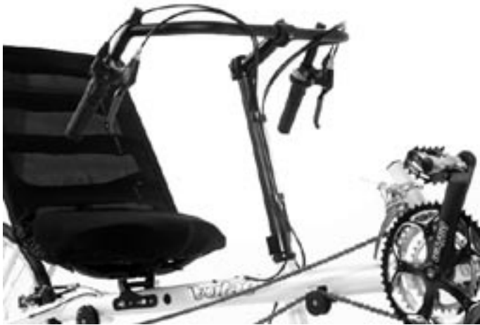
Volae Tour with the stock mesh back, slung foam base. The seat is the former Vision seat adapted to fit the Volae bikes. The Volae seat slide mechanism is one of the finest built today and really holds the seat on tight.
