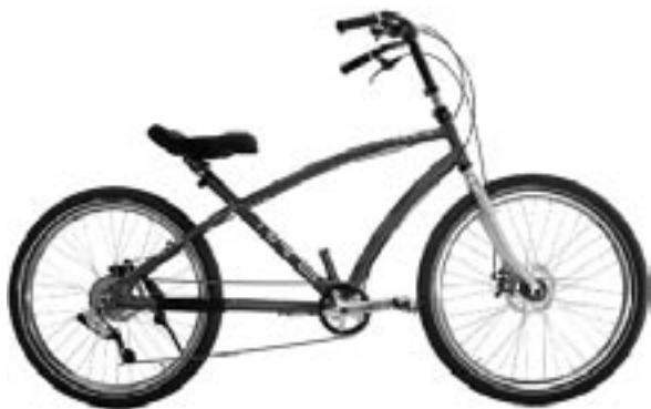
This is the RANS CITI. It has B-37 bars, Schwalbe Big Apple tires, a minimalist 9-speed drivetrain and disc brakes.
