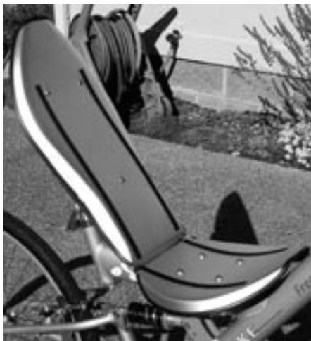
The Cruzbike's lightweight Aluminum shell seat.
