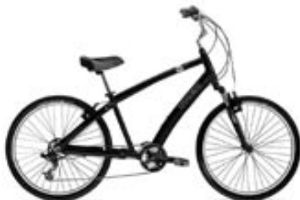
This is the 2007 Trek Pure Sport crank-forward. It has an Alpha aluminum frame, 21-speeds, V-brakes and sells for $460.
