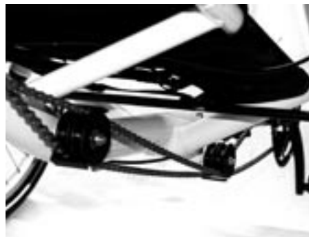
WizWheelz' chainline uses two double idlers and follows the line of the frame.
