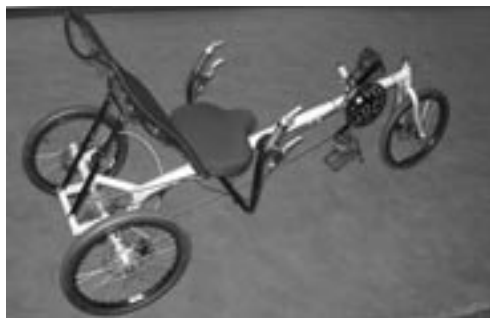
This is the prototype Greenspeed Frog. Note the proper differential (right) designed by Greenspeed's Ian Sims. This new 2007 model trike will have 16" wheels, disc brakes, a telescoping rounded square section frame.
