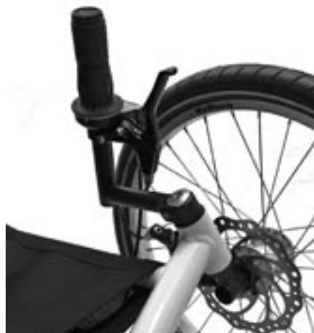
The Zoomer has "L" shaped direct steering handlebars somewhat like the Edge model.
