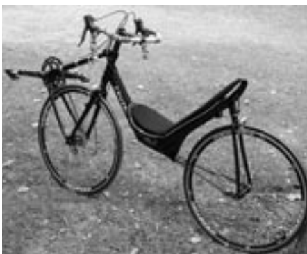
The lightweight Silvio has a carbon fiber frame, rear suspension and with light parts can weigh in the 23 pound range.
