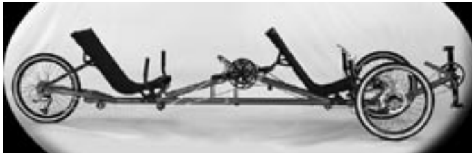
The WizWheelz tandem has S&S couplers for easier shipping. This is the most affordable of the tandem tadpoles.
