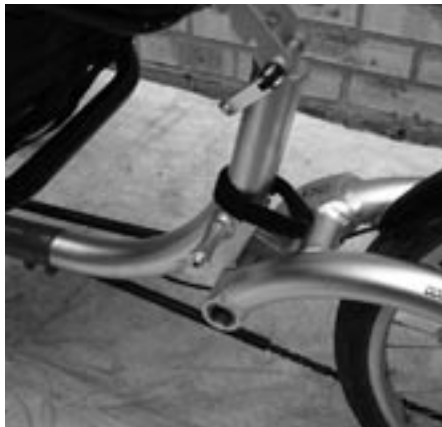
The rear swing arm, suspension pivot and seat mount.
