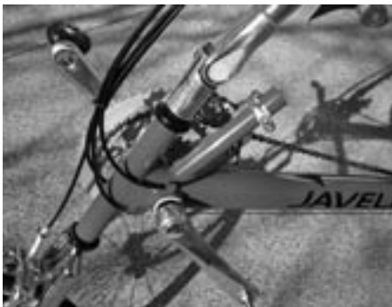
Forward frame section and adjustable stem — Alan Barnard
