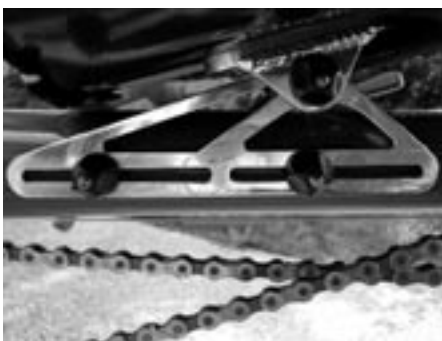
The quick-release seat slider Alan Barnard
