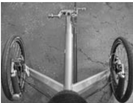
Note "Wing" cross-members allowing easy entry/exit
