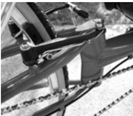
The rear triangle/main tube joint Alan Barnard
