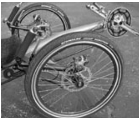
Front end: note radial spokes on the front wheel, Challenge hubs and direct steering
