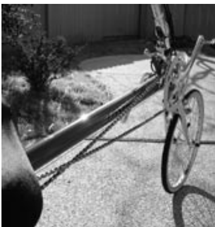
The main-tube. Note the much higher bottom bracket — Alan Barnard
