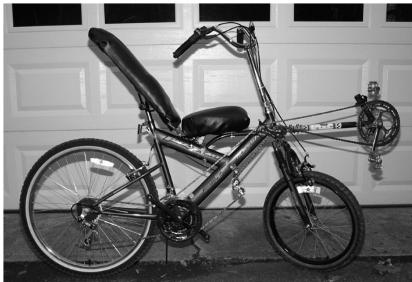
This is Tim Lipetz's no-weld Y-frame SWB (see No Weld #3)
