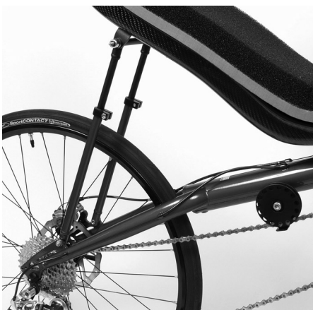
The robust telescoping seat stays offer infinite adjustment rather than matching holes with a ball-detent pin.
