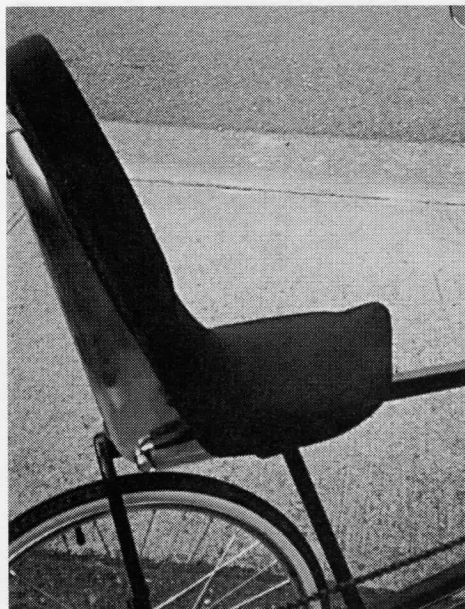
The new '96 EZ-1 seat has an aluminum shell with a foam base and back. The updated foam is higher quality, though the new lumbar makes rider sit more upright
