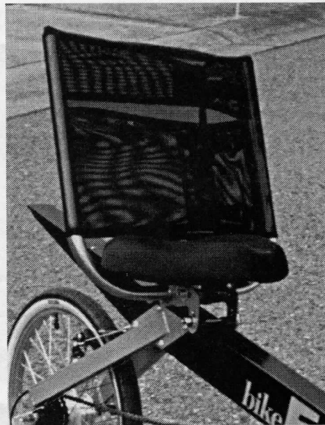
The '96 BikeE seat is a definite improvement and offers separate seat back/base adjustment.
