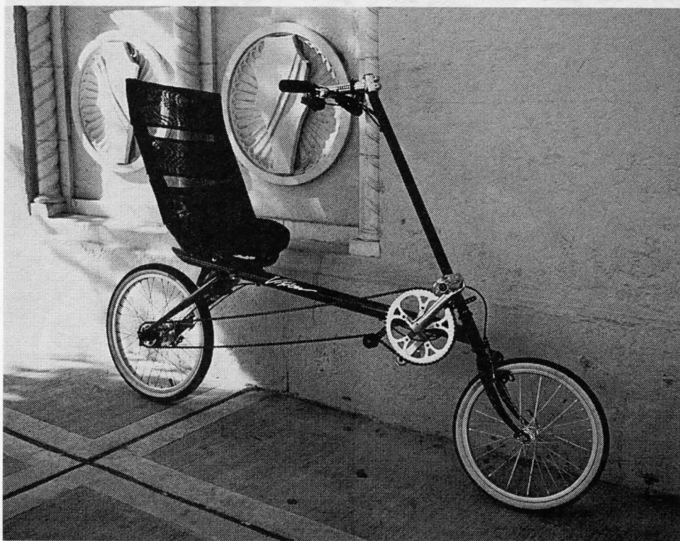
The Vision VR-30 "Metro" recumbent. The above bike is a prototype. The handlebars and stem have changed for the production version—courtesy of ATP Vision
